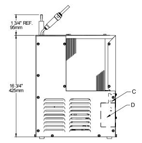
LEGEND A = 1/4" O.D. TUBE WATER OUTLET C = TEMPERATURE ADJUSTMENT B = 1/4" O.D. TUBE WATER INLET D = ELECTRICAL
