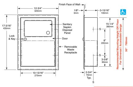
Rough Wall Opening 11-1/4" (285mm) wide 15-5/8" (395mm) high 4" (102mm) minimum recessed depth
